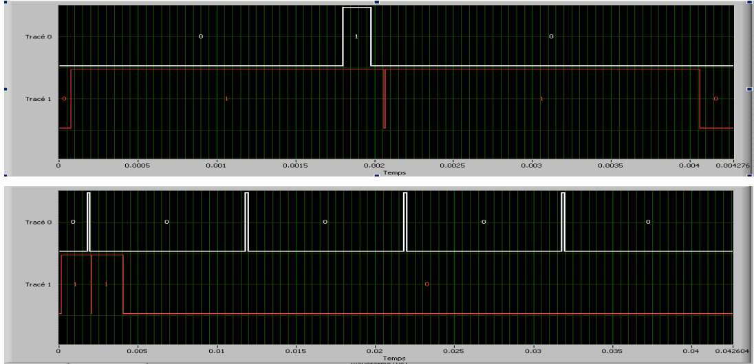
Figure 2.9: A typical pulse sequence for a stable discharge. The white traces and the red traces represent the pulse sequence for valve and discharge voltage. The upper-level of the white traces corresponds to opening time of the valve. The upper-figure shows a pulsed voltage DC glow discharge where the upper-level of the red trace corresponds to 0V and the lower-level corresponds to \sim -1000V . It is important to notice that, we apply the discharge pulse \sim 70\mu s later than the end of the valve pulse. The reason behind it is that, the mechanical constraint in the valve which not only makes a delay to begin the beam pulse but also changes the position distribution profile of the pulse. The lower-figure shows a discharge with multiple valve pulses in one valve-pulse sequence. In this case, the first valve-pulse is pulsed DC discharged while the others are continuous DC discharged.
