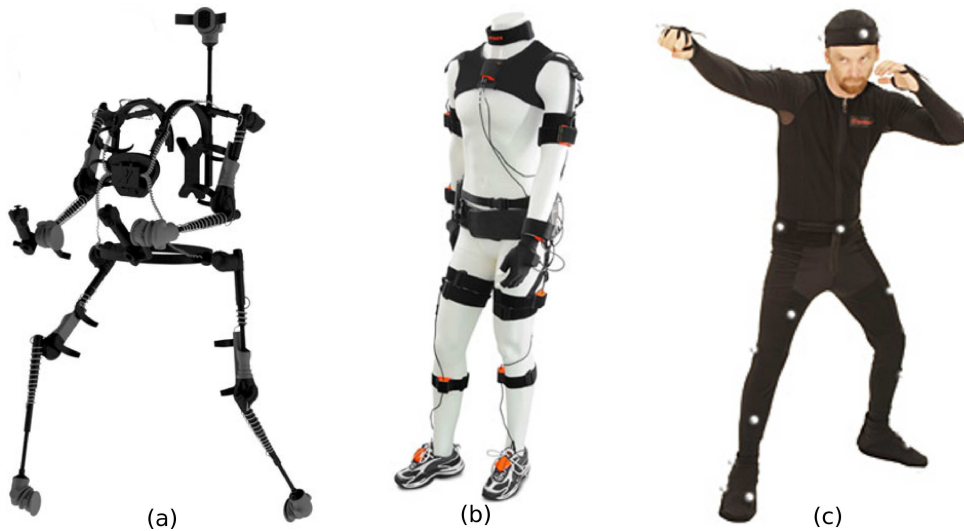
FIGURE 2.1: Examples of systems using markers. (a) exoskeleton of Gypsy ™ mechanical system. (b) markers of Xsens ™ inertial system. (c) markers of OptiTrack ™ passive optical system.
