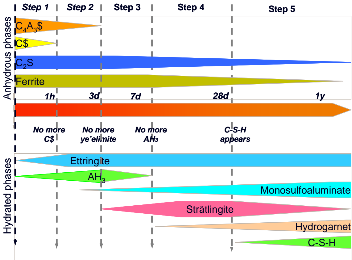
Figure 3-20: Steps observed during the hydration of k165-400B-5A in paste during the first year
