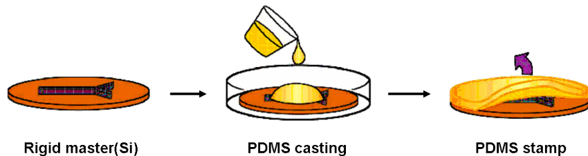
Figure 2.5: Schematic illustration of the basic procedure for the preparation of the soft stamp.
