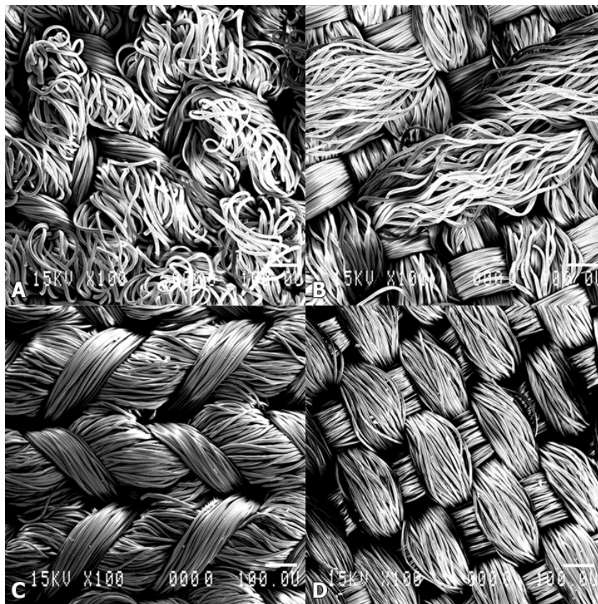
Figure 11: Scanning Electronic Microscopy images (SEM), showing the four textile structures (A: Biomateriali Knitted/velour, B: Biomateriali Woven/velour, C: Cardial Knitted and D: Cardial Woven). The lines at the bottom of the images correspond to 100 \mu\text{m} for 100X magnification.
