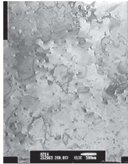
Fig. 2. Plan view TEM image showing the 5\text{--}7 \times 10^9 \text{ cm}^{-2} dislocation density.
