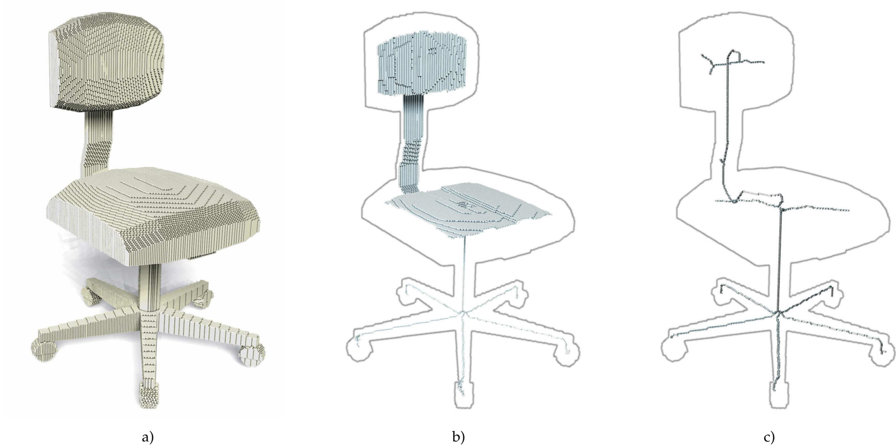
Figure 96: Chair - Homotopic thinning of a chair. a) , the original image (already presented before). b) , the result of DT3-2 algorithm (with the border of the original image superimposed). c) , the result of DT3-1 algorithm (with the border of the original image superimposed). The image continues on the next page.
