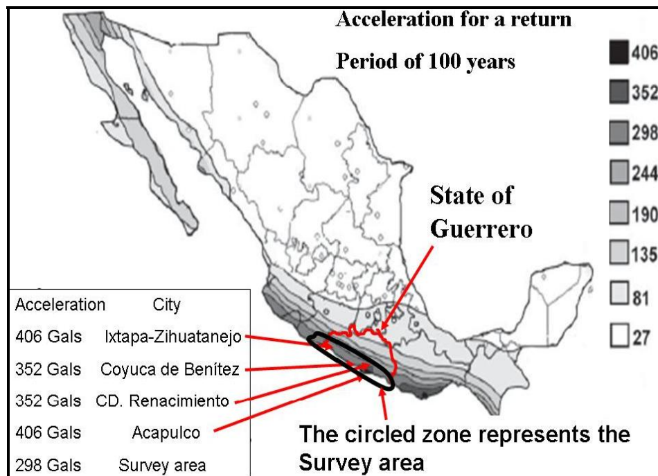
Figure 35 Maximum accelerations for a return period of 100 years [15].
