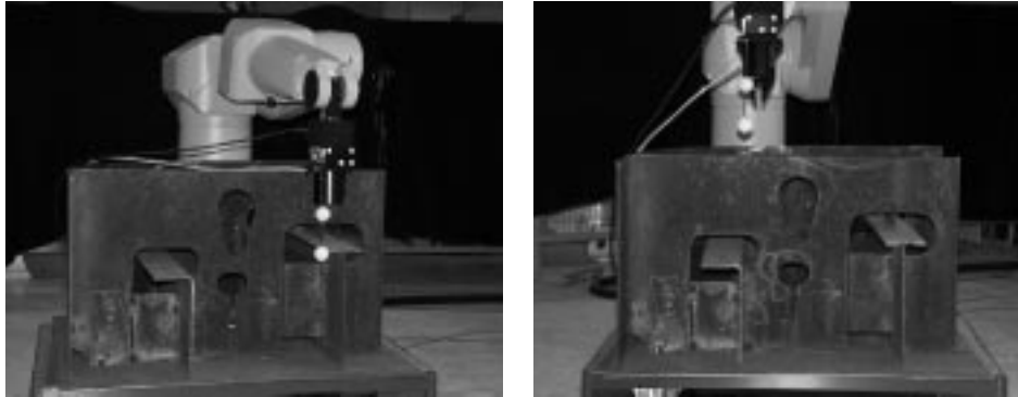
Figure 8.4: Projective encoding of set-points of alignment task: goal position (left), initial position (right)
