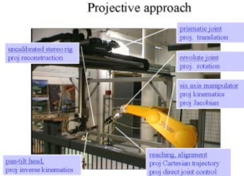
Figure 1.3: Modelling of a robotic work-cell using a stereo camera pair.
