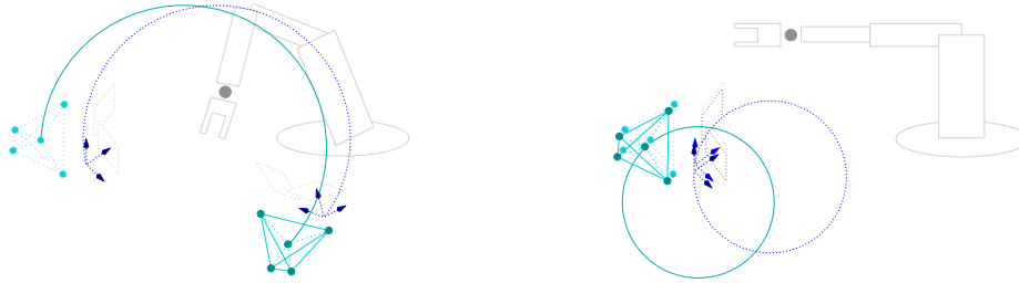
Figure 5.9: The projective kinematic mapping in a single projective frame, where the tetrahedron illustrates the projective camera frame associated with the stereo camera. Zero-reference and identical camera-motion (right). Robot-motion and apparent camera-motion, both projective (left).
