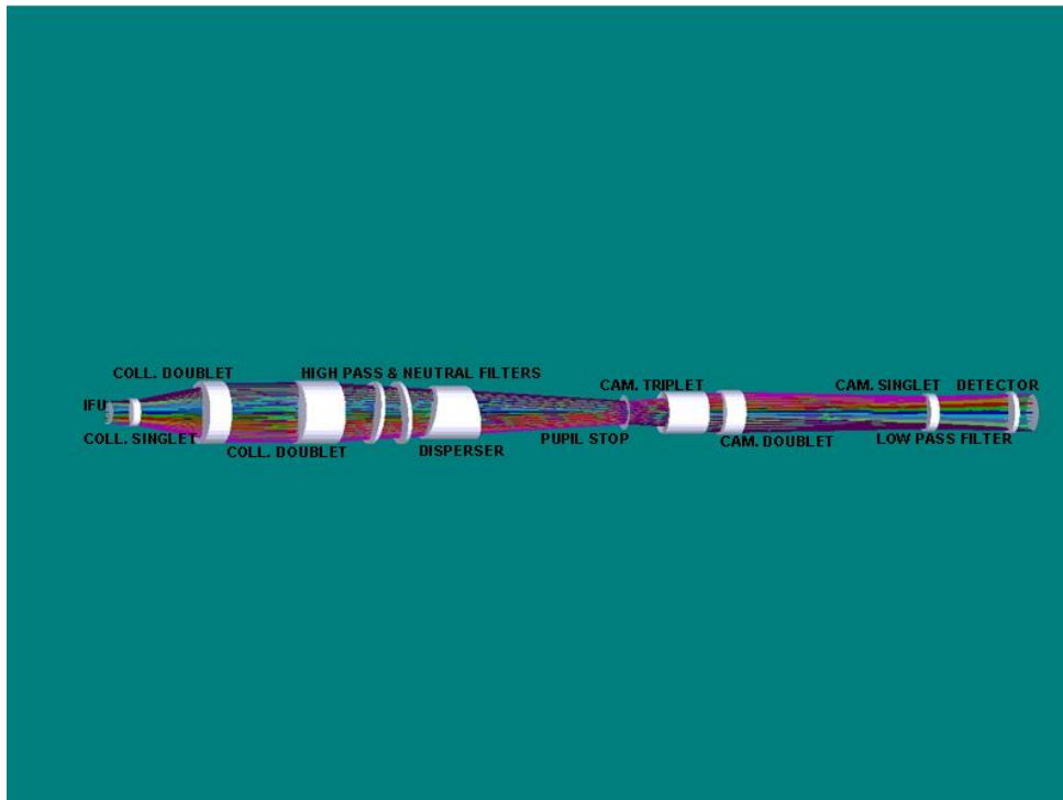
Figure 6-2: 3D-representation of the SPHERE Integral Field Spectrograph.
