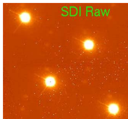
Figure 3-13: Raw images on the focus of NACO-SDI, by courtesy of the CHEOPS team. The simultaneous difference between them strongly attenuates the Speckle Noise.
