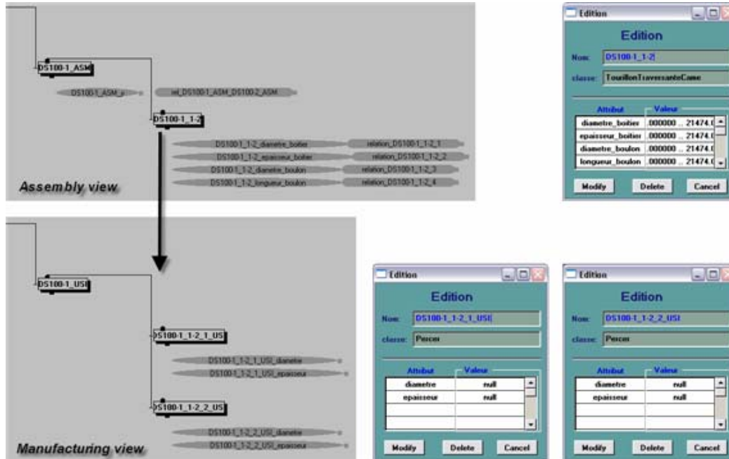
Figure 7.20 Example of assembly feature translation and propagation
