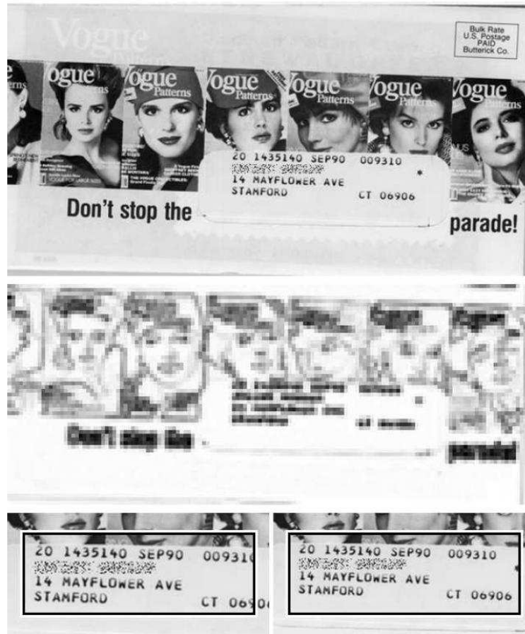
FIGURE 2.2 – A challenging sample file. As it can be observed, even after preprocessing there is still a large amount of background noise. While the left address candidate is almost correct the ZIP code is truncated. The right candidate (shown in the lower right) gives the complete address.
