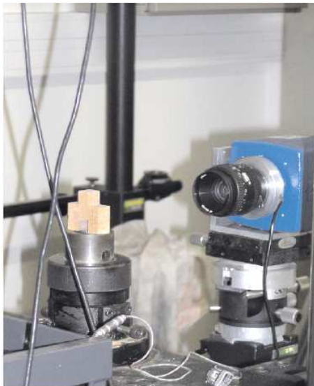
Fig. 6. Experimental device - testing machine coupled to a digital video camera.
