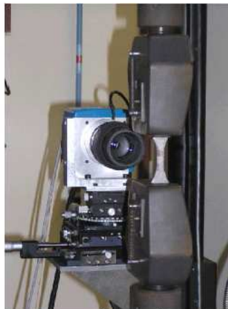
Figure 1 – Experimental setup: camera positioning and sample
