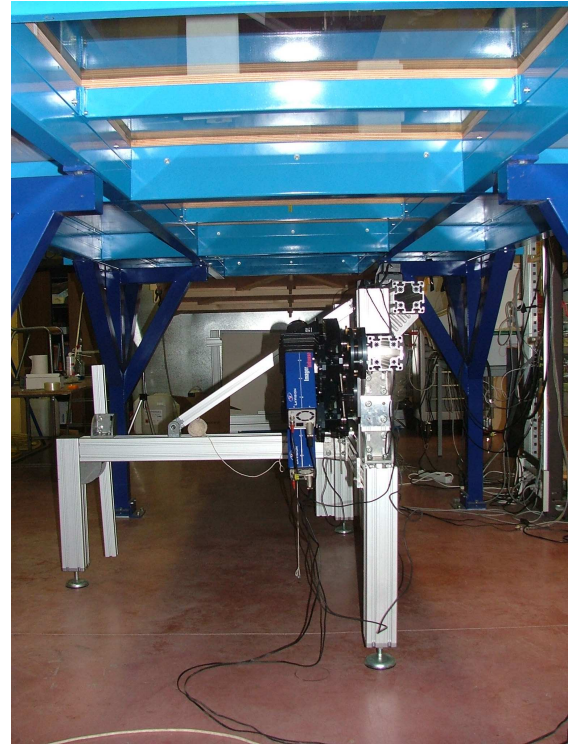
Figure 4.3: Side view of the stereo-PIV setup in the YZ configuration (LML)
