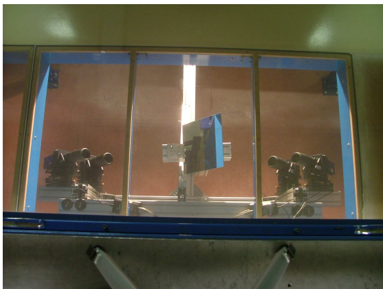
Figure 4.4: Stereo-PIV setup in the YZ configuration: view from the top of the wind-tunnel test section (LML)
