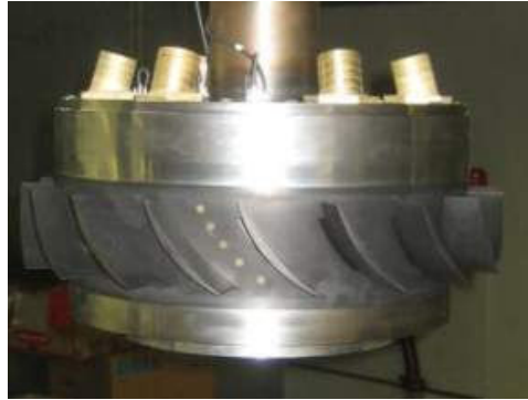
Fig 6.4: Static pressure taps on the hub wall of the stator blade row (Colombo et al. [36])
