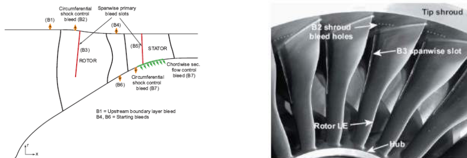
Fig 3.20 : Aspiration scheme of the fan stage (left) and the rotor (right)(Merchant et al. [11])
