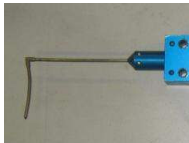
Fig 6.3: Aerodynamic probe (Colombo et al. [36])
