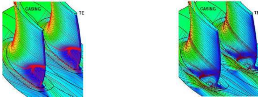
Fig 3.19: Stator surface Mach number contours and limiting streamlines without aspiration (left) and with aspiration by tailored OT (right) (Gümmer et al. [12])
