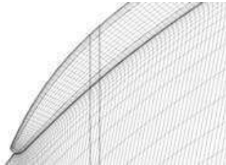
Fig 3.17a: Mesh of aspiration slot on rotor casing (Gümmer et al. [12])
