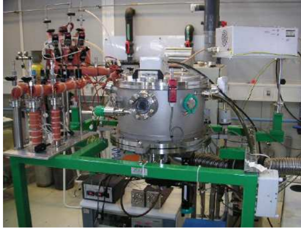
Figure 2-4. In-house built PECVD reactor for silicon oxide coatings.
