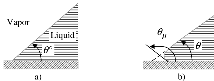
Figure 4-13. Contact angle of a liquid droplet: a) at 25° without any heat transfer and b) at saturation temperature on a heated surface: macro-contact angle \theta and micro-contact angle \theta_\mu .
