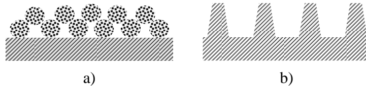
Figure 1-13. Illustration of cross section of: a) porous surface, b) rough surface.
