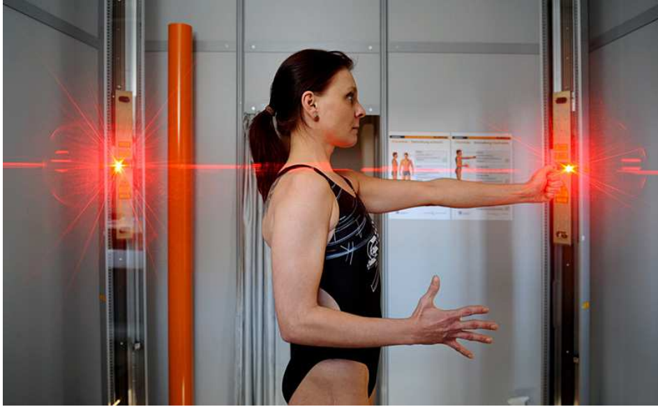
Figure 1.4: A Laser body-scanner : highly detailed surface geometry can be obtained by such scanners. Such detailed geometry is used for modeling textiles, medical analysis or for performance capture in the entertainment industry ©Human Solutions
