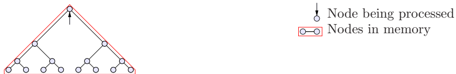
Figure 6.2: Memory state when the root node is being processed in a W1/R0 left-looking factorization. All the nodes have been loaded but none of them could be freed from memory.
