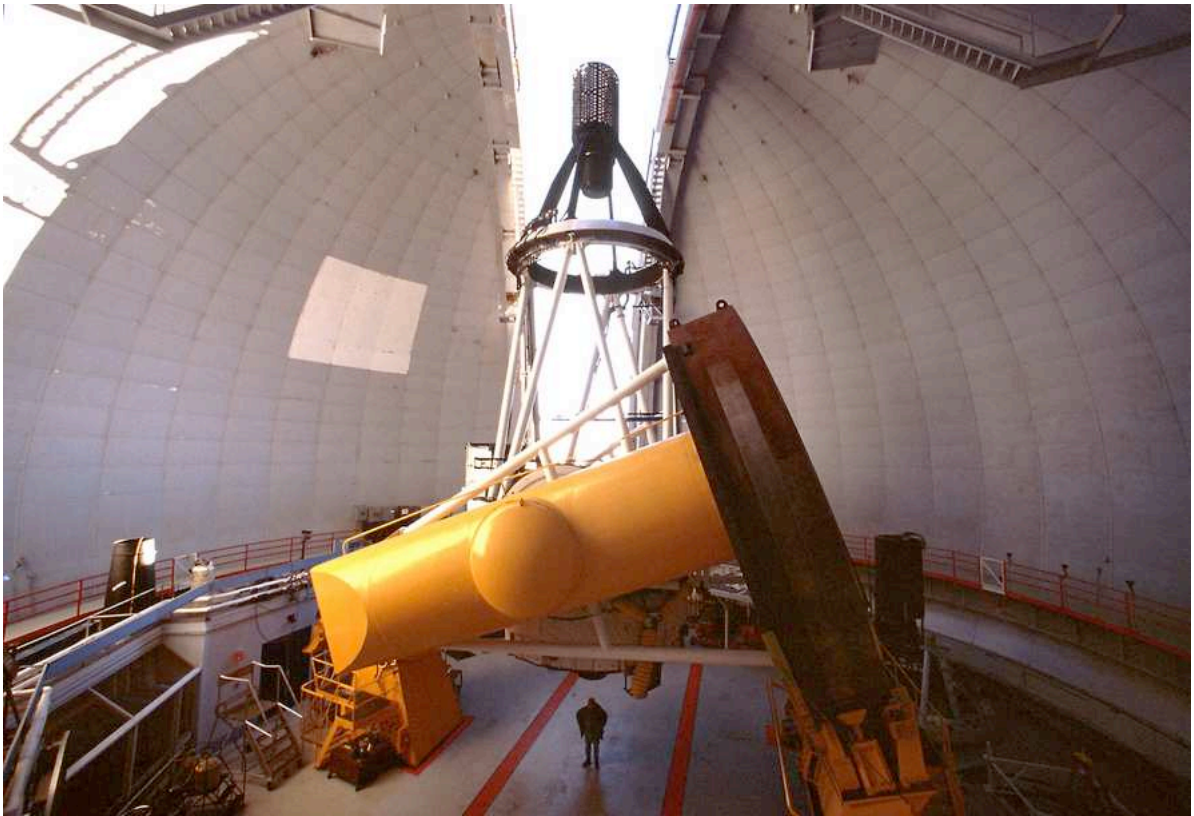
Figure 5.2: The MegaCam imager located at the prime focus at CFHT. Credit: CFHT homepage
