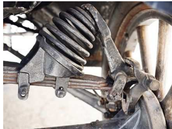
Figure 2.2: Model T Ford: leaf spring (left) and coil spring (right)
