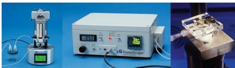
Figure II.9. Digital Instruments MultiMode microscope head with the thermal accessory installed (right); temperature controller (middle) and components of the thermal accessory assembled on the piezo-scanner (left).
