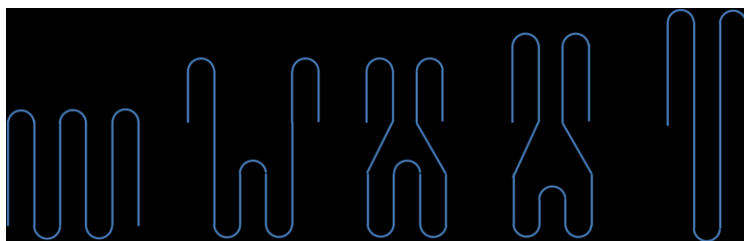
Fig. I.17: Schematic drawing of successive stages of the fold increase in single crystals on annealing.
