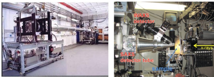
Figure II.8. Experimental hutch at the BM26 beamline showing the SAXS installation (left). The setup for the real-time simultaneous SAXS and WAXS measurements at beamline ID2 at the ESRF, Grenoble, France (right).
