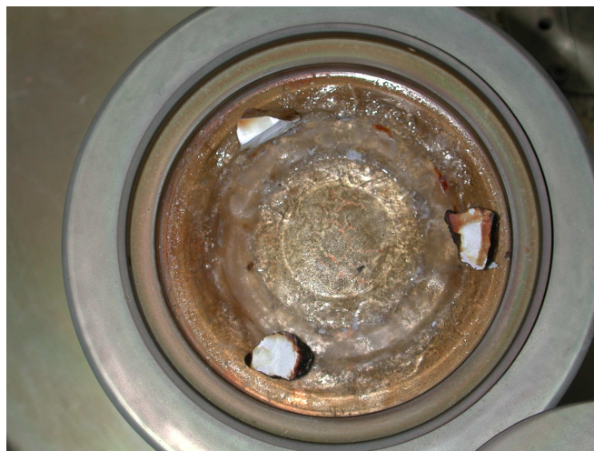
Figure III.16 : Photo de la cathode correspondante à Sr = 5%.
