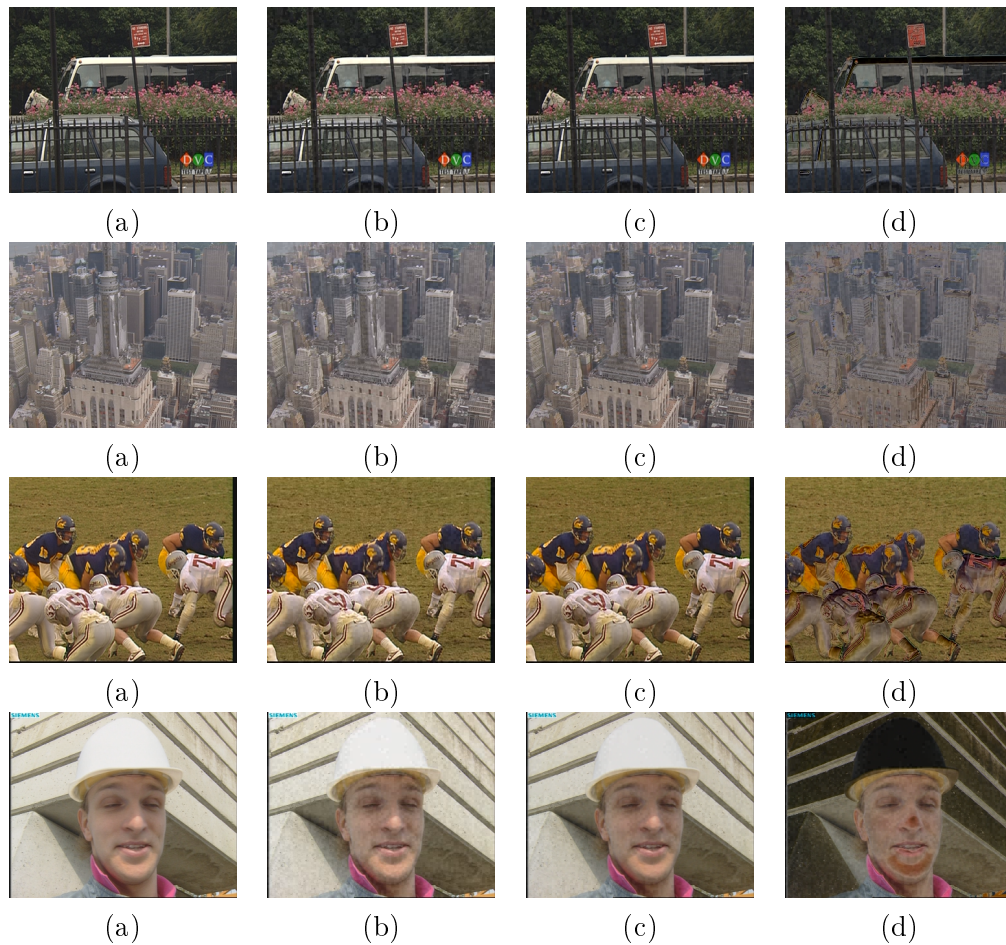
Figure 6.18: Colluded fingerprinted video sequences of bus , city , foreman and football : (a) Original frame, (b) Fingerprinted frame, (c) Average Collusion (17 colluders), (d) Modified negative collusion (8 colluders), ghost artifacts are prominent in video attacked by modified negative collusion with PSNR around 15 dB .
