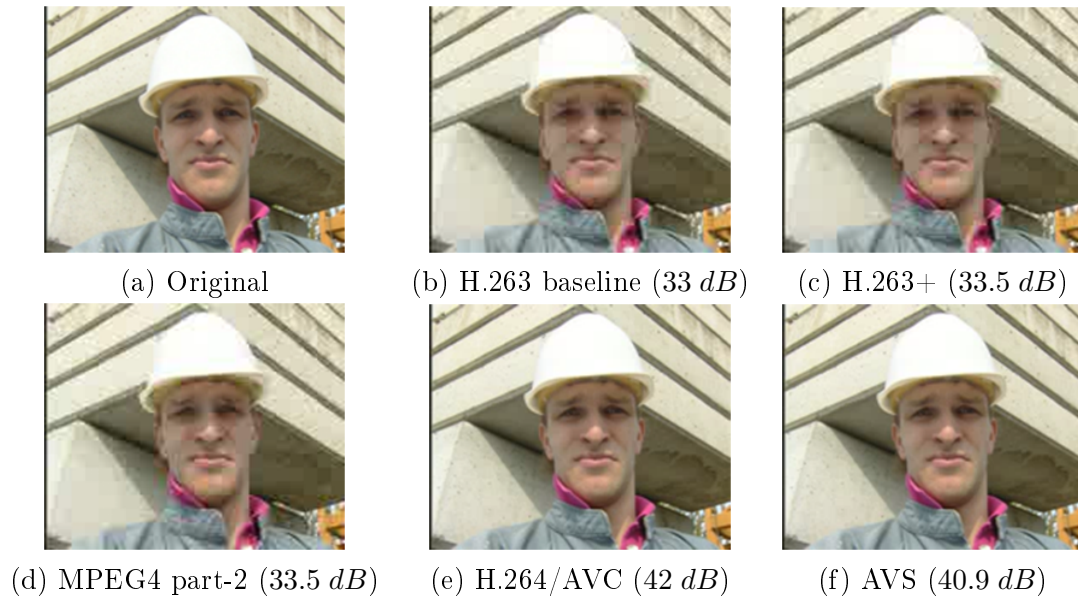
Figure 2.10: Comparison of H.264/AVC and AVS with previous video coding standards for QCIF resolution with 30 fps at 100 kbps.
