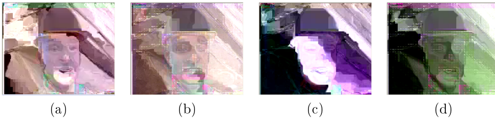
Figure 7.17: Attack in the selectively encrypted image by removing the encrypted data: (a) SE-CAVLC encrypted image \{Y, U, V\} = \{10.01, 26.86, 25.24\} dB, (b) SE-CAVLC attacked image \{Y, U, V\} = \{8.87, 27.3, 26.3\} dB, (c) SE-CABAC encrypted image \{Y, U, V\} = \{8.20, 17.95, 24.53\} dB, (d) SE-CABAC attacked image \{Y, U, V\} = \{7.72, 28.6, 24.6\} dB.
