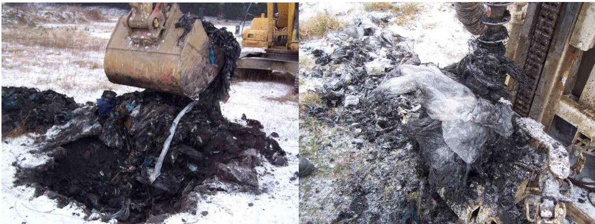
Figure VI- 31: Samples retrieved through shovel and boring.
