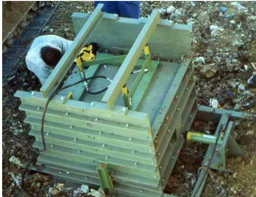
Figure VI- 3: Large scale in-situ direct shear box (Gotteland et al., 1995).
