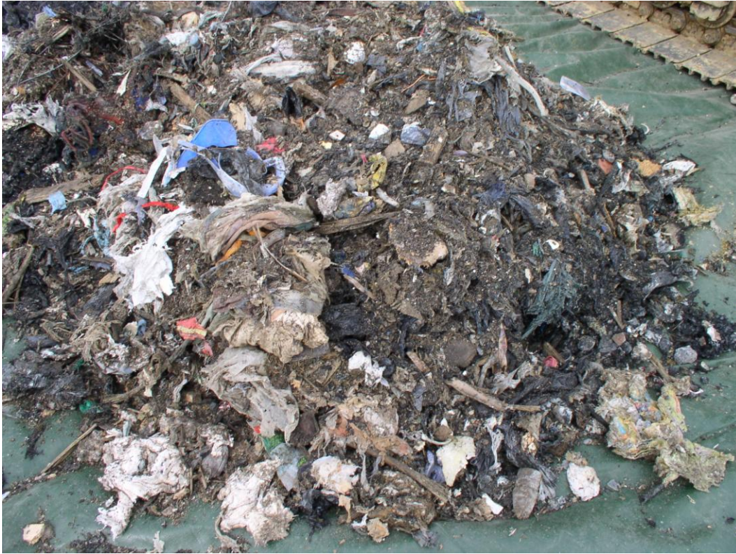
Figure VI- 43: Collection of waste from the drilling process for the in-situ density calculation.
