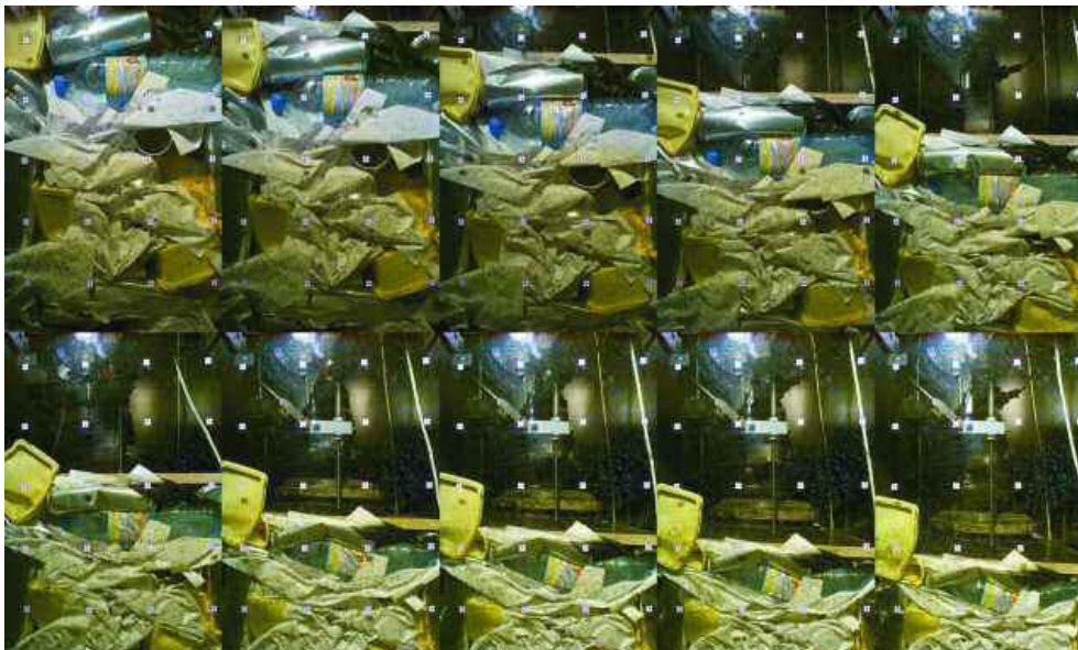
Figure II- 12: Compression of plastic components in the horizontal direction during the compaction of synthetic waste (Langer, 2005).
