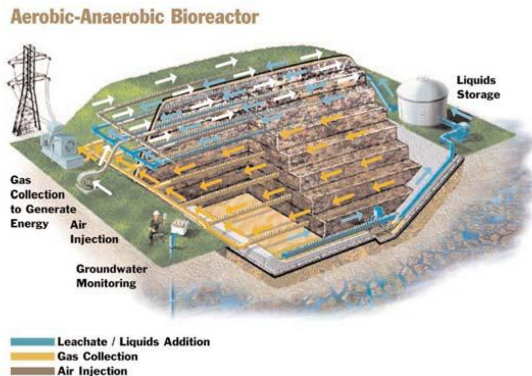
Figure I-22 : Hybrid bioreactor landfill (Waste Management, 2000).
