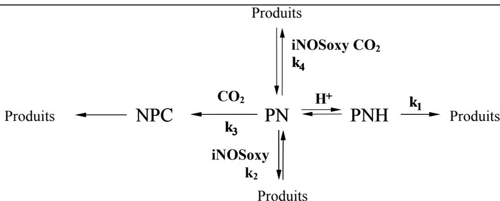
$$-\frac{d[\text{PN}]_t}{dt} = k_1 \times [\text{PNH}] + k_3 \times [\text{CO}_2] \times [\text{PN}] + k_2 \times [\text{iNOS}] \times [\text{PN}] + k_4 \times [\text{iNOS}] \times [\text{CO}_2] \times [\text{PN}]$$
