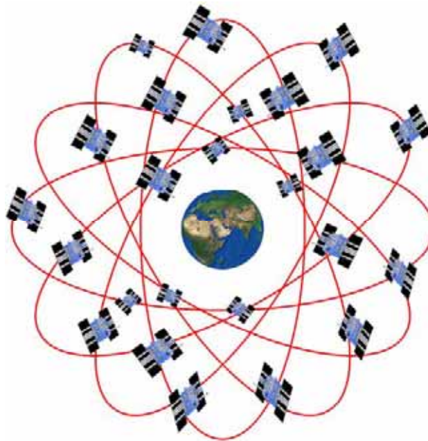
Figure II - 1 : Constellation des satellites GPS.
