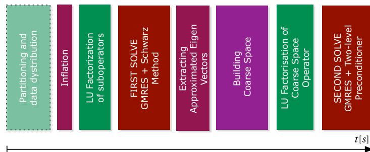
Figure 5.1: Stages of experiment 5.1 on time axis.
