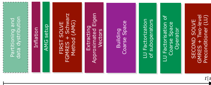
Figure 5.2: Stages of experiment 5.1 on time axis.
