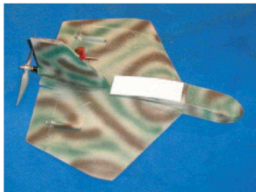
(a) Drone portable DO-MAV (EADS-Dornier, 42 cm d'envergure, 500 g)
