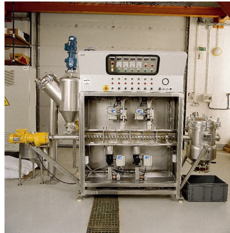
Figure 30: Batch and continuous microwave oven in industry
