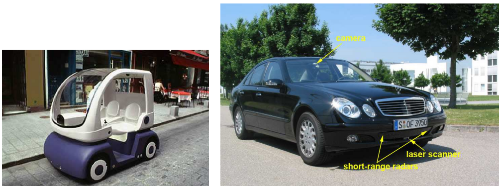
FIGURE 1.1 – Examples of intelligent vehicles : on the left, a cycab : experimental vehicle of INRIA and on the right, the Daimler demonstrator of european project PReVENT
