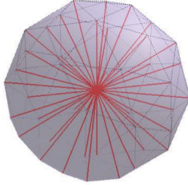
Figure 5.4: The red lines represent the directions for the normals from the origin, obtained by subdivided icosahedron.
