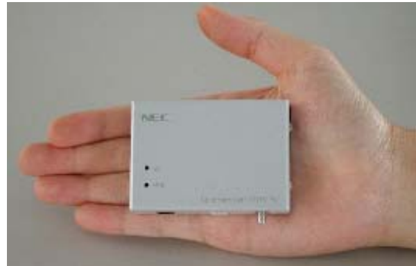
(b) Photo of encapsulated transceiver module
