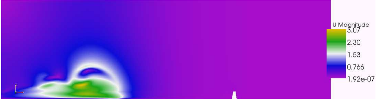
Figure 7.8: Velocity field magnitude at t = 25 s. The color scale ranges from 0 m/s to the maximum value 3.07 m/s.
