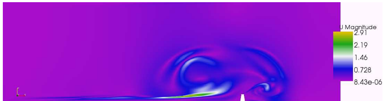
Figure 7.10: Magnitude of two velocity fields difference computed according to the standard and new models at t = 60 s. The color scale ranges from 0 m/s to the maximum value 2.91 m/s.
