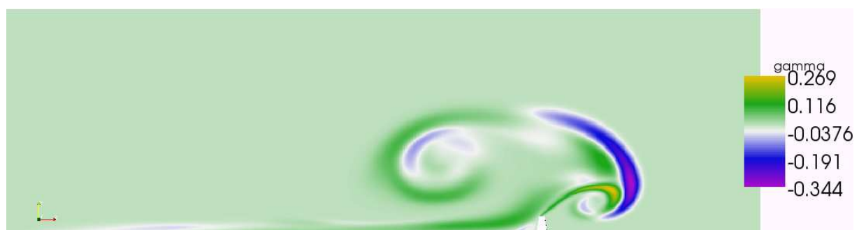
Figure 7.11: Difference of the volume fraction distributions computed according to the standard and new models at t = 60 s. The color scale ranges from -0.344 to the maximum value 0.269.
