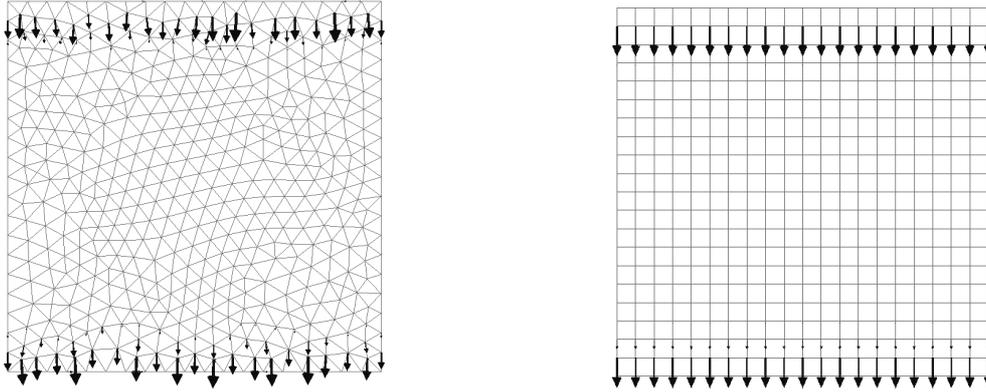
FIG. VII.1 – Exemple de vitesses parasites,  $|\mathbf{u}_h^1|_{L^\infty(\Omega)} = 1.16 \times 10^{-3}$
