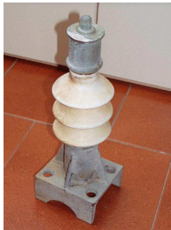
Figure 4.10. The 3 kV DC isolator used in the experimental characterization attempt (courtesy of RFI, Italy); attention was paid to ensure good ohmic contacts at the two extremities.
