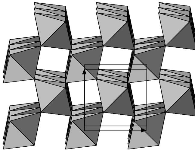
Figure I-6: structure de  $\beta\text{-MnO}_2$  (pyrolusite)
