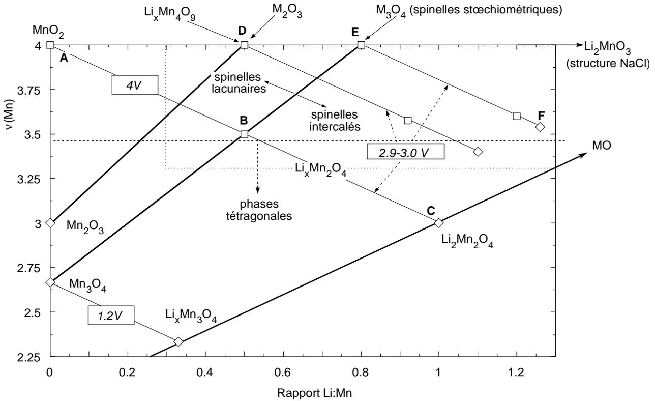
figure III.5: diagramme composition-valence Li-Mn-O pour les valences  $2.25 \leq v(\text{Mn}) \leq 4$ . 4. A:  $\lambda\text{-MnO}_2$ , B:  $\text{LiMn}_2\text{O}_4$ , C:  $\text{Li}_2\text{Mn}_2\text{O}_4$ , D:  $\text{Li}_2\text{Mn}_4\text{O}_9$ , E:  $\text{Li}_4\text{Mn}_5\text{O}_{12}$  <sup>27,32</sup>.
