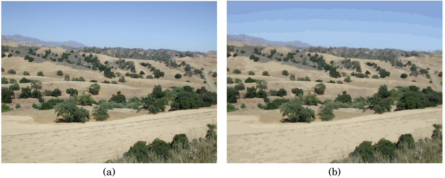
Figure 11.6: (a) Source image (b) Each pixel is given the color of the mode it converged to during the mean shift segmentation.
