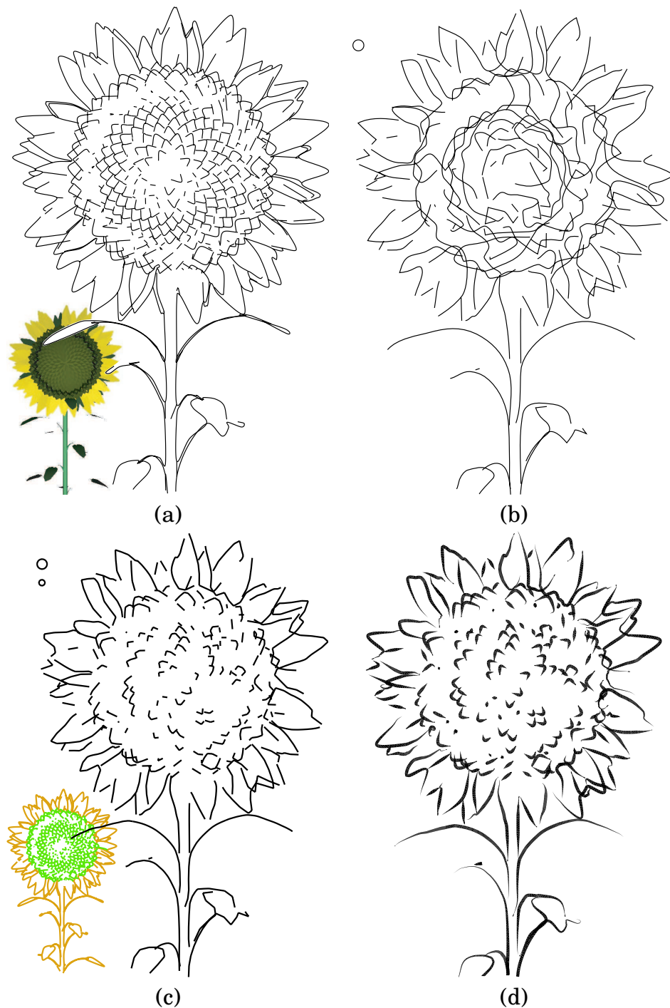
Figure 7.10: Simplification of a 3D rendering: (a) 3D model and its line rendering using silhouettes and suggestive contours (531 input lines) - (b) Simplification without any category (256 clusters) - (c) Using two categories (external and internal contours) each with a different scale and geometric strategy (294 clusters) - (d) Same result in a calligraphic style.
