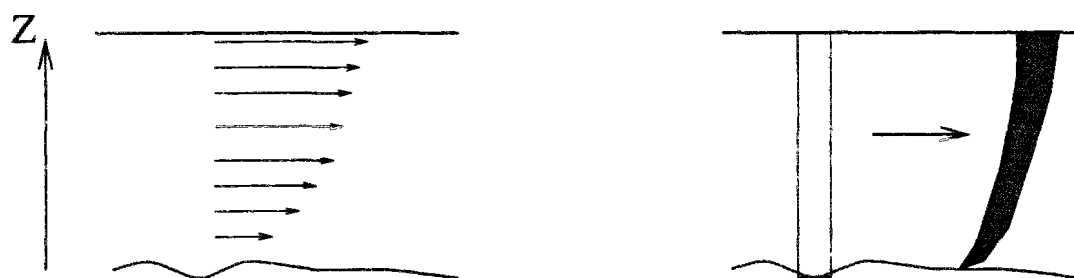
Figure 11.9: Main mechanisms causing longitudinal dispersion
