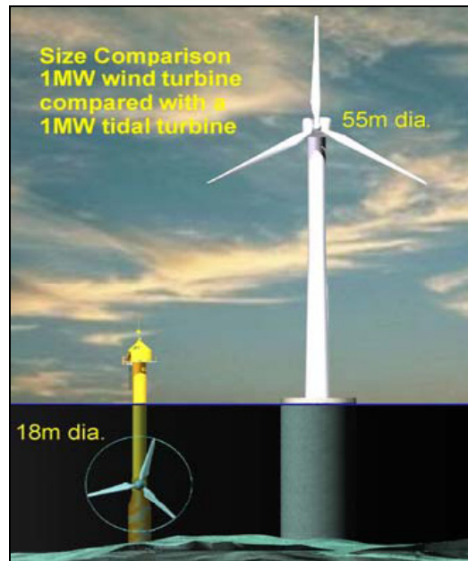
Fig. I.5. Tidal turbine against an offshore wind turbine [© MCT].
