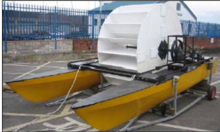
Fig. I.25. The University of Southampton completed tidal mill [41].
