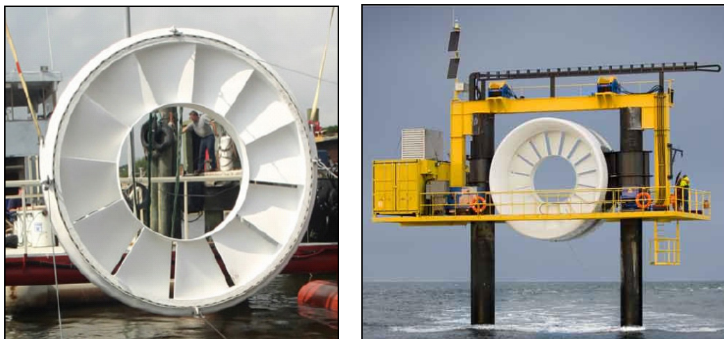
Fig. I.13. The Open-Centre turbine [© OpenHydro].
