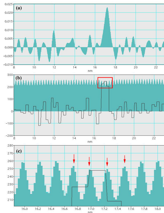
Figure IV-18: \epsilon_{zz} strain within the GaN WL measured by GPA (a) and the projection method (b). In Figure (b) the strain scale is multiplied 10^4 times and superposed on the HRTEM image profile. Figure (c) is an enlargement of the zone shown by the red rectangle. Red arrows indicate the contrast decrease within the GaN WL.
