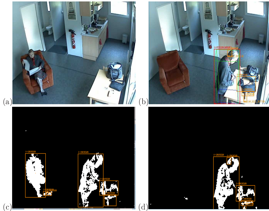
Figure 5.7: The effectiveness of removing background regions misclassified as person. At the beginning, the person sits in the armchair (figure (a)). Then she moves to the table (figure (b)) and this is the first time the camera can observe the region of the armchair. If we do not verify person blobs, the controller thinks that the armchair region is a person and it requests the background subtraction algorithm not to update this region. The results is illustrated in figure (c). With the verification of person blobs, the controller understands that the detected foreground region at the armchair is not a real person, it requests the background subtraction algorithm to update this region normally. Therefore, this foreground region disappears after several frames (70 frames in case of the algorithm EGMM). The results are illustrated in figure (d).
