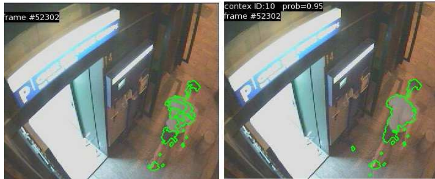
Figure 2.14: The sample of detection results of the original codebook [Kim 2005] (image on the left) and the context-based codebook [Martin 2008] (image on the right)
