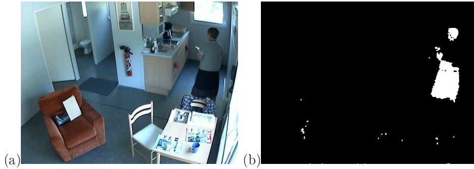
Figure 6.25: The background subtraction algorithm fails to detect the chromaticity of the person coat is similar to the chromaticity of the wall. Image (a) is the original image. Image (b) is the detection results.
