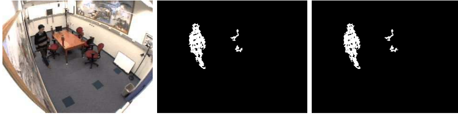
Figure 6.14: The detection results using different homogeneity constraints on “Intelligence room” from project ATON [ATON]. The left image is the original image, the middle image is the detection results of 2PC. The right image is the detection results of 3PC.
