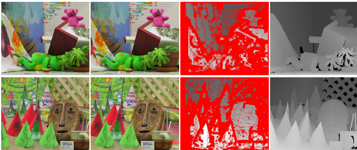
Figure 4.4: From left to right: Reference and secondary images, estimated sparse disparity map and ground truth. On top: Teddy. On bottom: Cones.
