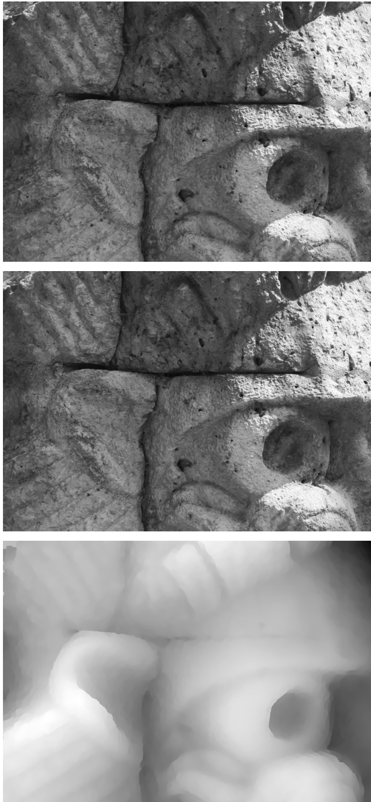
Figure 6.15: “Lion” experiment. Reference image. Secondary image. Disparity map (100% of points after median of the blocks).
