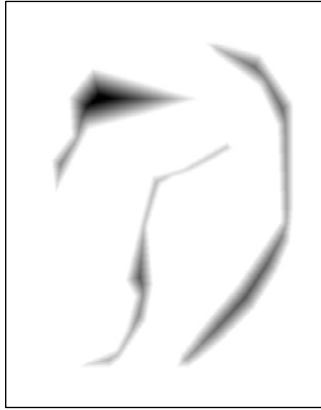
Figure 20 The Euclidean Distance Map (EDM) of the image in Figure 16. The darker the grey of shade, the longer the distance.
