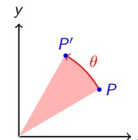
$$\begin{pmatrix} x' \\ y' \end{pmatrix} = \begin{pmatrix} \cos \theta & -\sin \theta \\ \sin \theta & \cos \theta \end{pmatrix} \begin{pmatrix} x \\ y \end{pmatrix}$$
