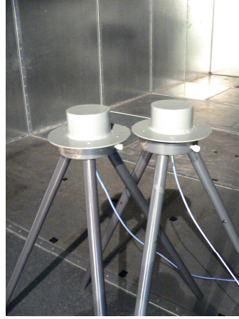
Figure 2.33: The interior of the reverberation chamber with two conical monopole antennas
