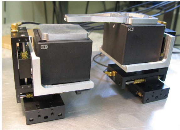
Figure 4.7: Illustration of the first AFM prototype.
