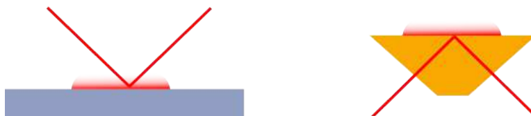
Figure 2.3: Total Internal Reflection and Total Reflection illumination methods.
