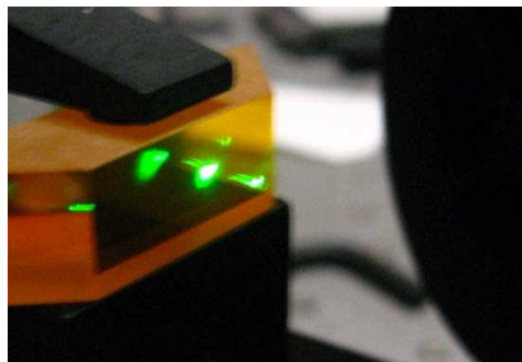
Figure 5.6: Projection on the sample of the green light source at the detector position.
