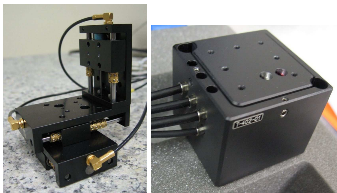
Figure 4.5: From left to right - three inertial translation tables assembled together; piezo scanner with 1nm resolution in closed loop.
