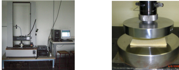
Figure 86. Machine de traction/compression INSTRON 33R4204
