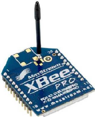
Figure C.11 – XBee Pro Module with whip antenna
