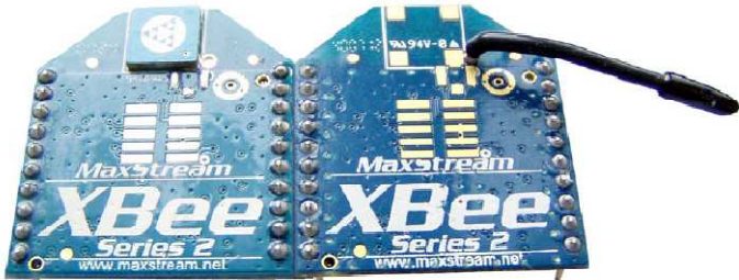
Figure C.11 – XBee Pro Module with whip antenna
