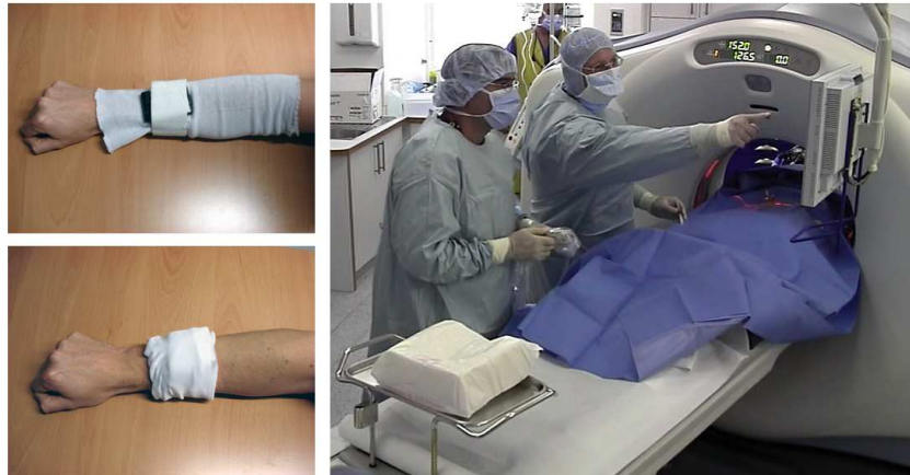
Figure A.1: (Left) Attachment of the inertial sensors with bandages. (Right) Setup during a vertebroplasty procedure.
