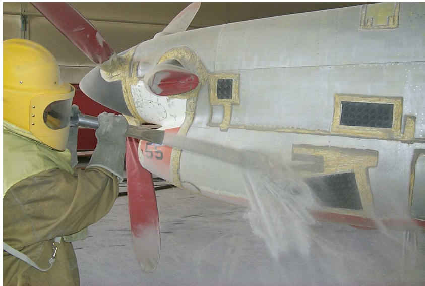
Figure 4. Fuselage stripping of T-25 aircraft at PAMA-LS.
